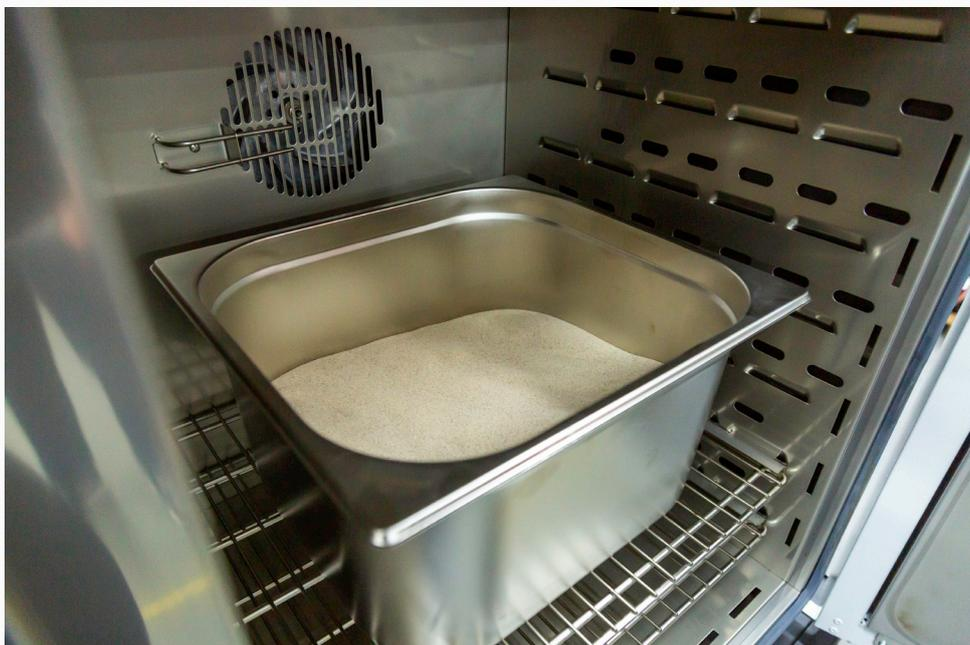
After 3 hours, the temperature must be increased to 200 °C / 392 °F for the next 5 hours. Both temperature cycles should be performed with air circulation system on.
