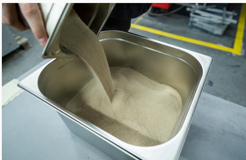
After the printing is done and the printing chamber has cooled down to room temperature, the models need to be removed from the build plate and placed in a metal container filled to roughly 10 mm height with quartz sand with a grain gradation of approximately 0.6 mm.
