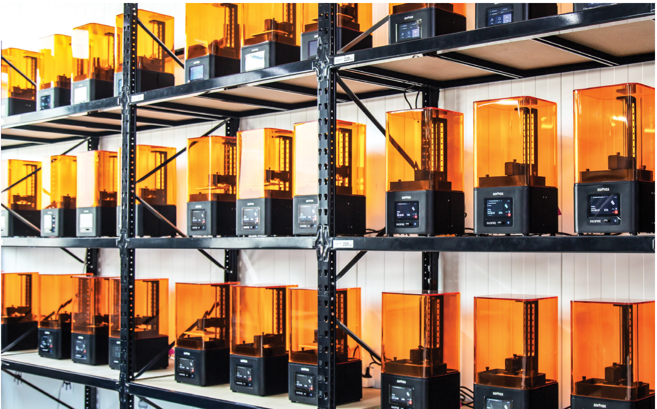
A farm of 30 Zortrax Inkspire 3D printers can offer 650,000 to over 1,000,000 parts of monthly output.
