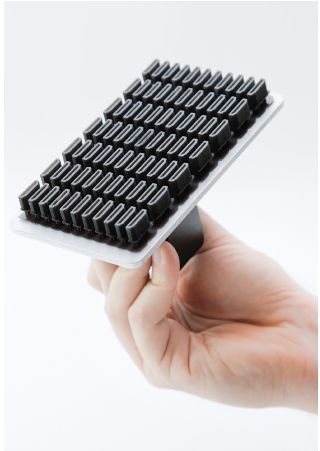
77 HDMI cover caps 3D printed on Zortrax Inkspire in 51 min.
