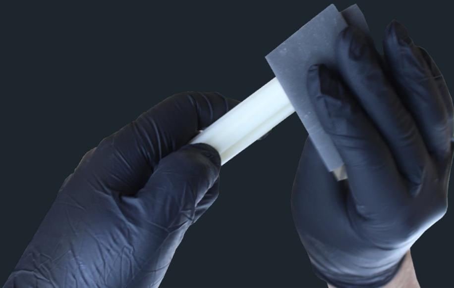
**TIP** | If you decide to try various abrasive techniques, remember that sanding and sandblasting should be performed before glass bead blasting, as they are more abrasive and can leave fine scratches on the surface which can be further removed by glass beads.
